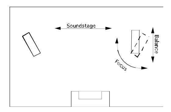
In blind listening tests the preferred angle turned out to be 72° with the listener at the apex. However, the optimum angle depends on the dispersion pattern of the specific type of speaker.
