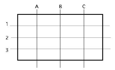
Referring to the above example, the cross points 2A and 2C are the ideal starting position for speaker placement. Place the listening chair at B less than 3 feet from the wall. This represents the seating arrangement in the first diagram.
