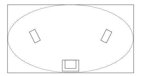
So why did we place the listening chair near the rear wall? The first reason is bass reinforcement. Maximum sound pressure occurs at the room boundaries and pressure gives the sense of deep bass. Secondly, because the reflections off the rear wall are shorter than the circumference of the head, the brain cannot measure the time delay between the ears. If it cannot measure the time delay it cannot localize the source of sound. When the brain cannot localize reflections it ignores them.
